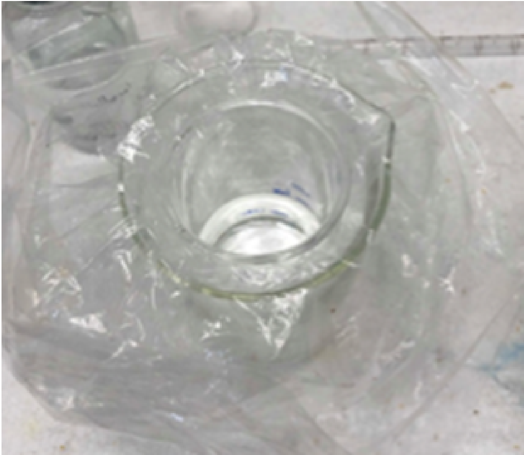
Figure 1: Beaker Set Up for Transferring Fire Ants into Hexane Solution. A plastic bag was placed inside of a 250mL beaker. A 150mL beaker, containing hexane and water, was placed within this setup.
